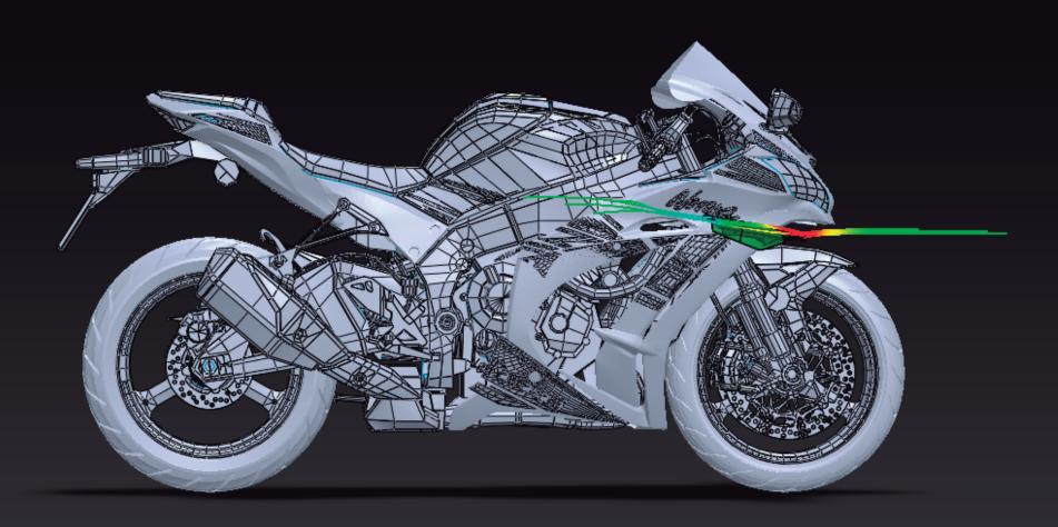
The Spoiler gives aerodynamic pressure at the front section of the bike, improving dynamic performance.
