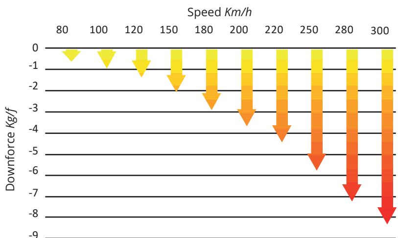
The Downforce that the spoilers generates raises potentially as the speed increases, at 300 km/h we get 8.3 Kg/f.
