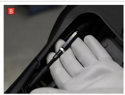
Before fitting the Scorpion slip-on system the original valve needs disconnecting and the Scorpion servo wheel requires fitting.
