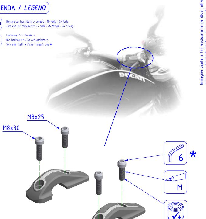
\* PER IL SERRAGGIO DELLE VITI RIFARSI AL MANUALE DEL COSTRUTTORE FOR THE TIGHTENING OF THE SCREWS REFER TO THE MANUFACTURER'S MANUAL
