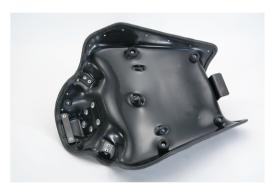
2. Lift the stock seat up and back to remove from motorcycle.
