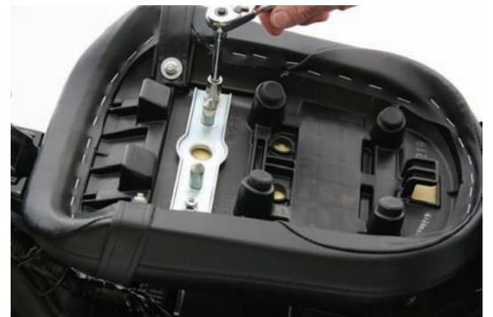
4. Install stock mounting bracket onto bottom of Mustang seat using the supplied bolts.
