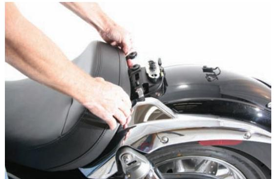
3. Turn rear seat over and remove stock mounting bracket. It must be transferred to the Mustang seat.
