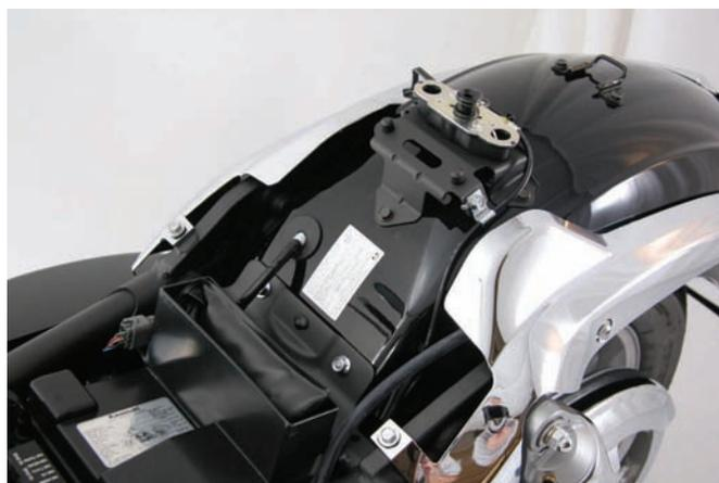
3. Engage tab on front of Mustang seat onto frame. Push center of seat down onto key-latch bracket until it clicks into place
