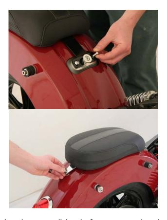
3. Holding the solo seat parallel to the frame, engage the solo seat's rear bracket with the fender stud.
