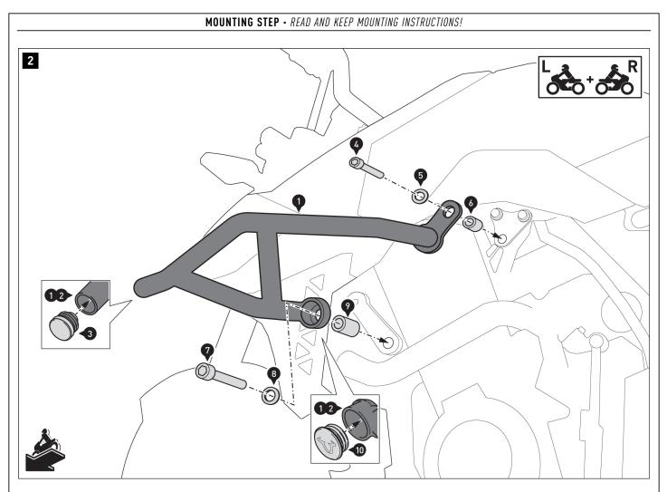
Insert the plastic plugs (3) into the openings of crash bars (1) and (2).
