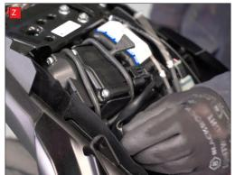
Y) Disconnect the cables from the motor.
