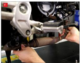
H) The supplied spring washers and nuts can now be used to hold the header in place. Do NOT fully tighten them at this stage.
