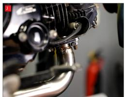
I) Line the hole in the mounting bracket up with the original mounting point on the frame and then screw the original mounting bolt in a couple of turns.
