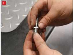
I) Remove the original fitting from the foot peg. Do not open or move the foot peg whilst this fitting is removed.
