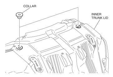
39. Clean the surface of the area shown using isopropyl alcohol.
