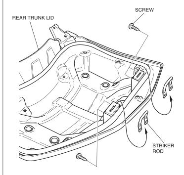
29. Remove the inner trunk lid as shown.
