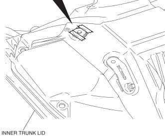
41. Install the inner trunk lid to the trunk lid as shown.
