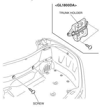
13. Remove the front trunk lower panel as shown.
