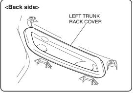
34. Clean the surface of the area shown using isopropyl alcohol.
