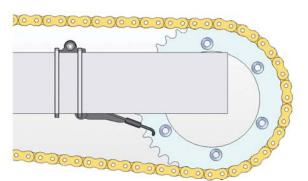
The injectors should lie in line with the chain, but not resting on it. Remember to allow for play in the chain. The injector tips should rest at about the '7 o'clock' position on the sprocket. Nibs should rest against sprocket face angled slightly inwards, but pointing downwards.
