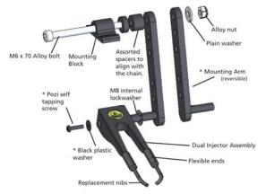
The adapter kit combined with the Dual Injector kit will allow fitting to certain models.
