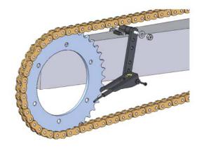
Hold the mounting block with bolt on the top of the swingarm and insert spacers on the M6x70mm alloy bolt to achieve alignment with the chain using lock washers between any two plastic surfaces.
