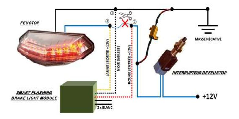
Access the brake light components and disassemble to access the electrical wires. There are two wires leading to the stop light. One is the ground wire and the other is a power wire (+12 V when the brake is used). Now you need to determine which wire is the ground wire and which wire is the power wire. Use a voltmeter or refer to a wiring diagram. In most cases, the ground wire has a black or brown color.
