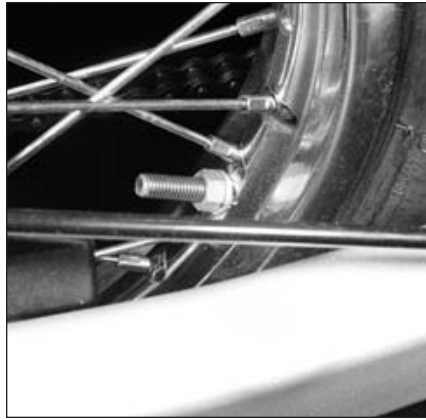
5.7 Tighten the locknut on the rim lock to the specified torque
