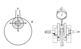
Measure the misalignment on the journal bearing of the crank shaft.
