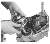
Detach a kick-starter spindle, shift-fork shaft and shift fork.
