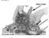
Detach a stud bolt, guide plate, generator and parts. Have the crankcase processed by a motorcyle specialist shop.
