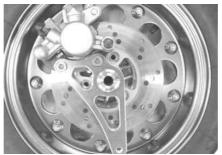
Install and tighten the caliper to a caliper bracket with an M8x12 socket cap screw to the specified torque.
