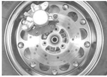
Install the caliper to the disk rotor Install the disk rotor.
