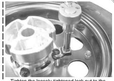
Tighten the loosely-tightened lock nut to the specified torque.
