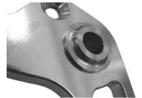
Change the sleeve of the caliper bracket with the supplied one.
