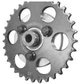
Install and tighten, to the specified torque, the driven sprocket to the retainer COMP. with the supplied lock nut, and install the collar.
