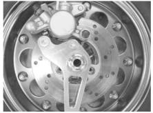
Install and tighten the caliper to the caliper bracket with a flat head screw to the specified torque. ▲NOTE: Be sure to always follow the specified torque.
