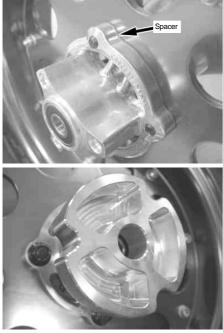
Sandwiching the wheel between wheel hub assembly and dumper hub, tighten them, loosely for now, with a supplied lock nut.
