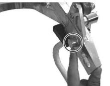
If the swing arm, installed on your motorcycle, is a standard type, cut off the panel stopper on the axle holder.
