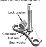
cone races, and then attach steel balls to the cone race.
