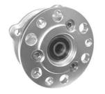
with the supplied disk bolt and lock nut, and tighten the disk rotor to the specified torque. Torque: 25 N · m (2.5 kgf · m)
